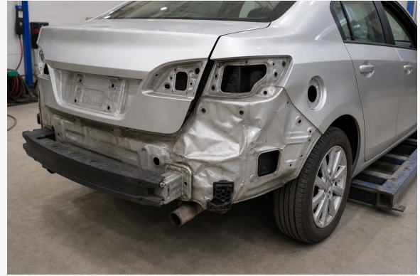
Figure 2. Illustrative pre-repair view with exterior components removed, showing damage to the rear body-panel area and adjacent unibody structure.
